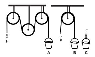
In which of the given situations, the force F needed to lift a bucket of water is the least?
