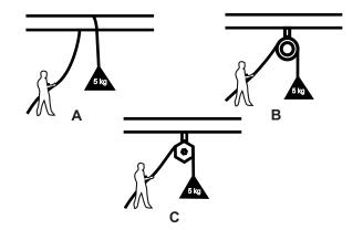
A man is lifting a mass of 5 kg. In which of the given figures, does he apply the minimum force?
