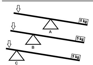
In which one of the given figures, minimum force will be required to lift 5 kg?
