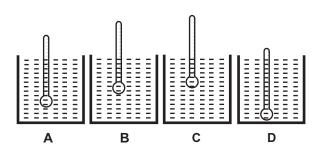
In which of the given figures, a lactometer would indicate the maximum water impurity in milk?
