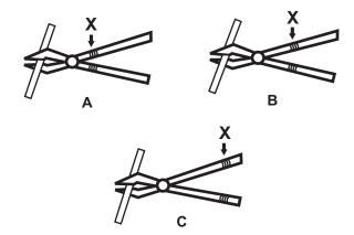
In which one of the given figures, the force is required to cut the wire will be minimum if force is applied at X?
