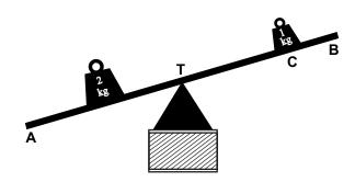
Where should the smaller weight be shifted from C to balance the beam on fulcrum at T?
